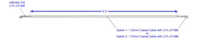
R-SMA with Install Heat Shrink Tubing Or Option 2- 1.37mm Coaxial Cable with U.FL-LP-088 and Hex Nut
