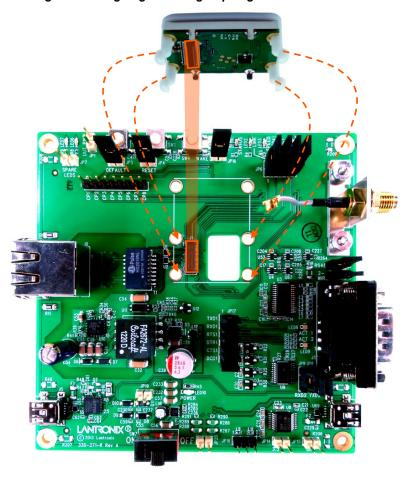
Figure 3-2 Aligning Mounting Clip Legs to Standoff Holes
