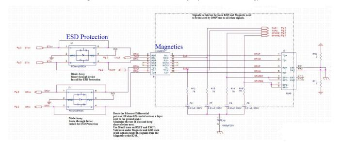
Figure 2-7 Ethernet Connection Example (xPico wired unit only)
