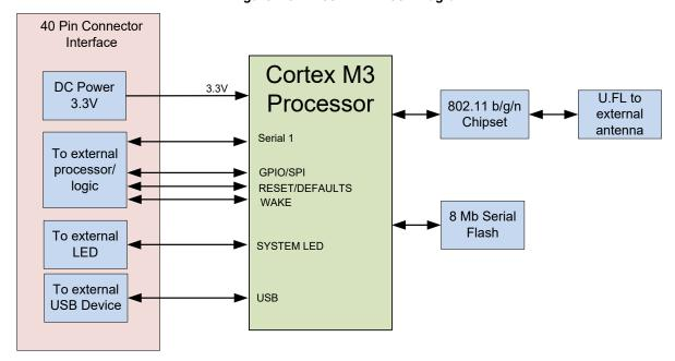
Figure 2-3 xPico Wi-Fi Block Diagram
