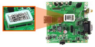
**Note:** When removing the xPico embedded device server from the evaluation board, gently tug the module. Do not use excessive force or attempt to remove the xPico module by grasping and pulling the module from the short end opposite the module connector as this may cause damage to the J1 evaluation board connector.
