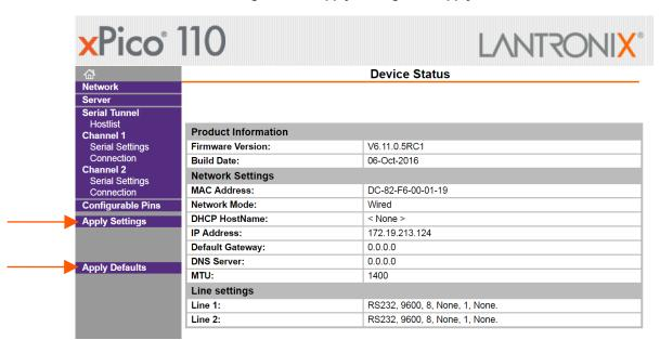
Figure 4-10. Apply Settings and Apply Defaults
