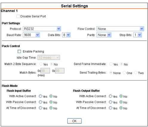
Figure 4-6. Channel Serial Settings
