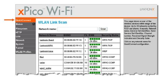
6. Upon selection of the **QuickConnect** option, the xPico Wi-Fi device scans and displays up to 20 wireless devices in order of strongest signal strength at the top.
