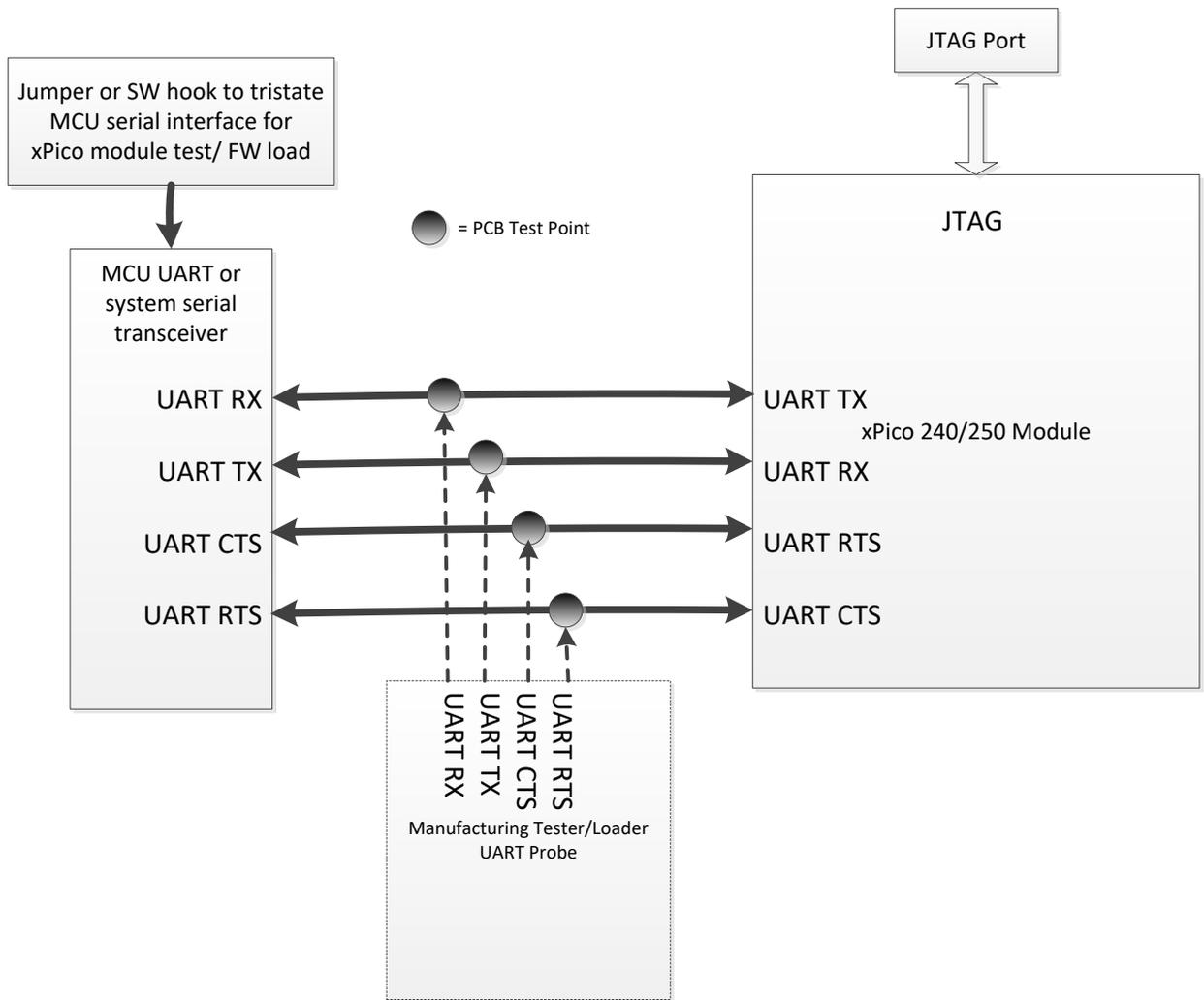
See the evaluation board schematic and artwork for recommended transceiver, DB9, and port connections in the [xPico 200 Series Evaluation Kit User Guide](#).
