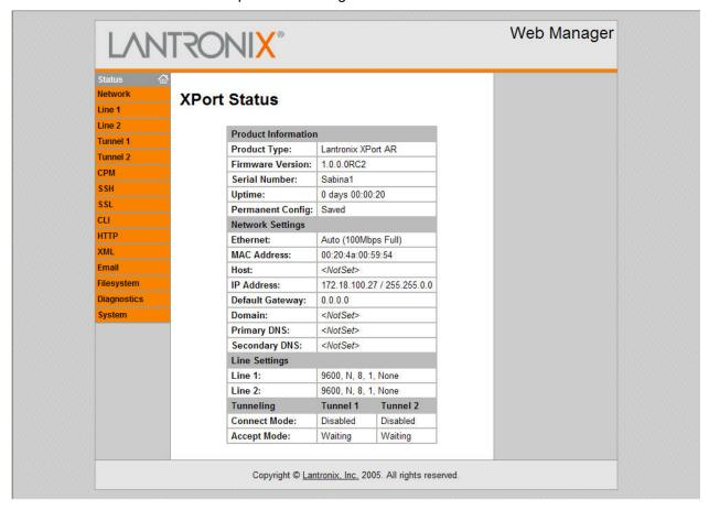
3. Use the menu to navigate to sub pages where you can configure the XPort AR. Unless otherwise noted, changes are applied immediately to the XPort AR.
