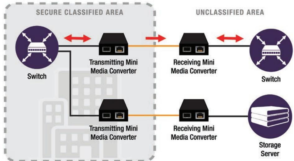
The second diagram illustrates a secure network that needs to be updated with data from an unsecure external source, where it can be analyzed and used to make key decisions. Unidirectional communication ensures no data is able to leave the classified area.
