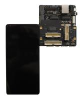
The display expansion board includes a FHD+ AMOLED display with capacitive touch panel along with audio connectors, sensor GenX connector, Legacy sensor connector, 20p JTAG connector and front camera card connector.
