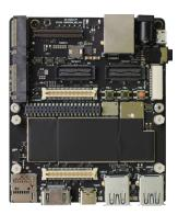
The Snapdragon 888 main board measuring 100mm x 85mm, is where all the processing occurs.
