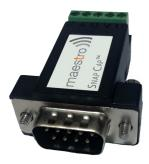
SNAP CAP<sup>™</sup> RS-485 converts Lantronix M110 or E210 series' RS-232 port on a 9-pin sub-D connector (female) into an isolated half-duplex or full-duplex RS-485 port on a 5-pin, 3.5 mm pitch, COMBICON connector.
