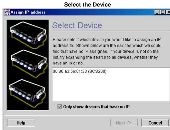
3. Select the SCS that appears in the window and click **Next**. The Assign IP address - Assignment Method Select window displays.
