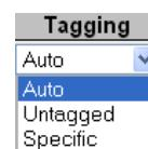
**Auto:** causes the software to automatically find a VLAN ID that will match the ECE. VLAN ID will be the lowest in the range of matching VLAN IDs (except 0 (priority-tagged), unless the ECE only matches priority tagged traffic). If the ECE only matches untagged traffic, no tag will be inserted in the generated traffic.
