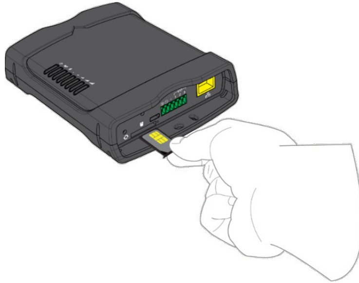
Figure 5-3 Inserting the SIM card
