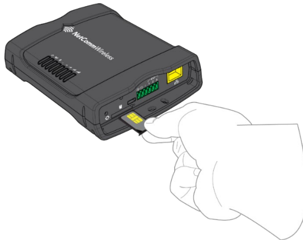
Figure 5-4 Inserting the SIM card
