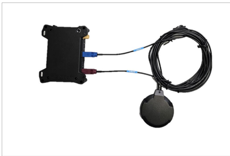
Figure 8: Connecting the external antenna
