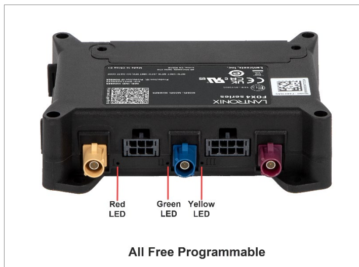
Figure 19: View of LED indicators
