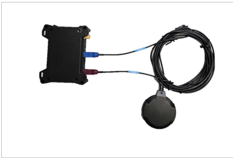
Figure 24: GSM/GNSS External antenna connected to FOX4-4G device
