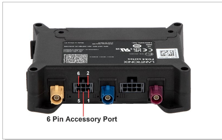
Figure 13: Pin Assignment of 6-pin Accessory Port
