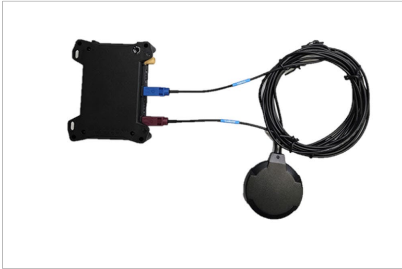
Figure 24: GSM/GNSS External antenna connected to FOX4-4G device
