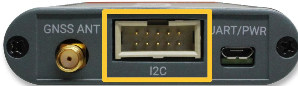
**Figure 8. I2C and Power Measurement Connector**
