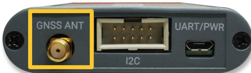
**Figure 7. GNSS SMA Connector**
