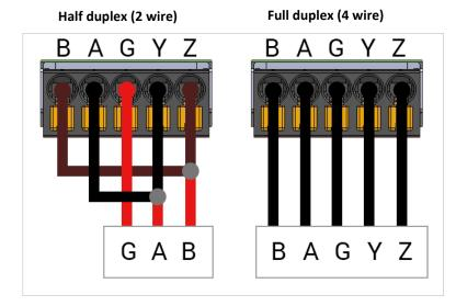
Figure 2-9 RS-485 Wiring Diagram
