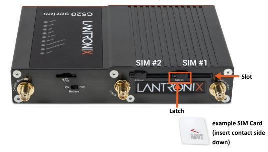
Figure 2-5 Dual SIM Operation
