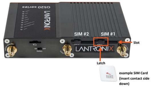
2. Gently insert the SIM card (contact side down) into the slot and push to lock it in place. Release the latch.
