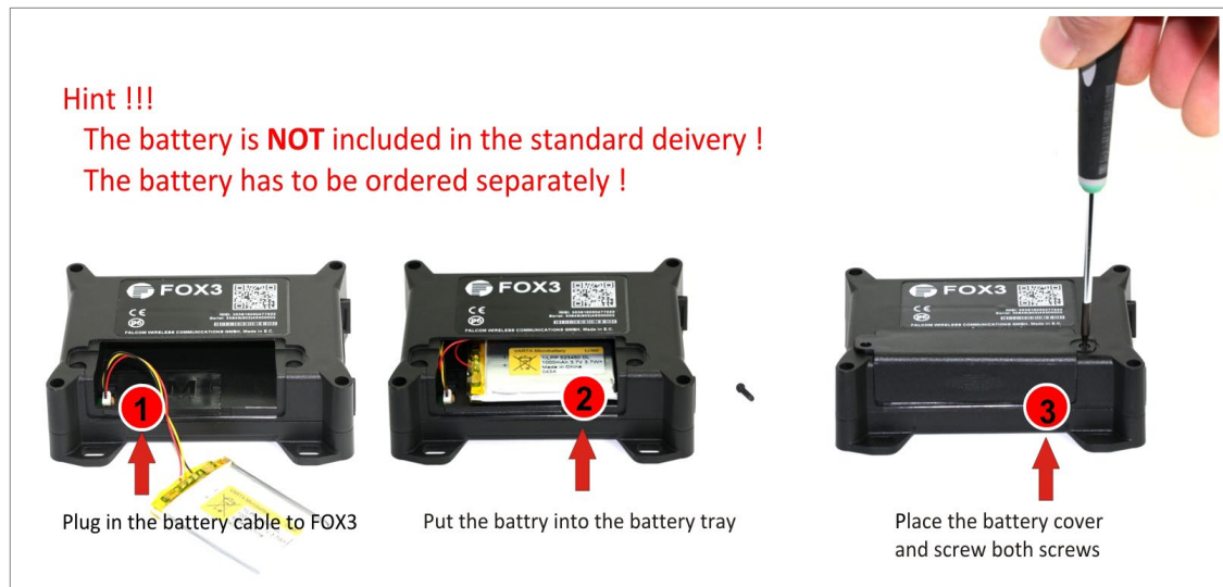
Figure 14.1: Connecting the battery to the FOX3-2G/3G/4G devices
