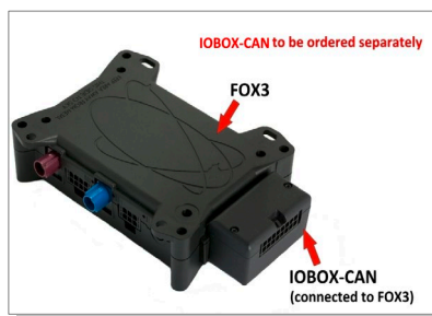
FOX3-2G/3G/4G with IOBOX-CAN/WLAN plugged in
