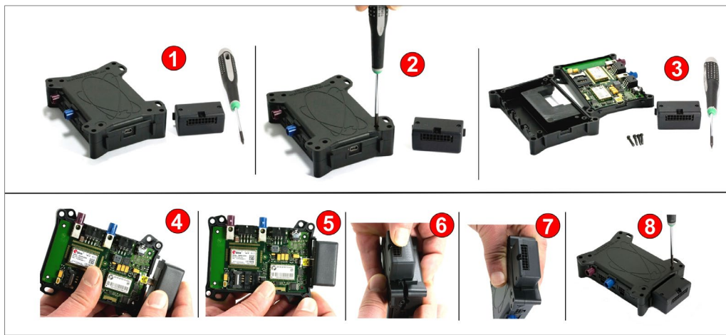
Figure 22: Mounting IOBOX-MINI or IOBOX-CAN/WLAN to the FOX3-2G/3G/4G devices.
