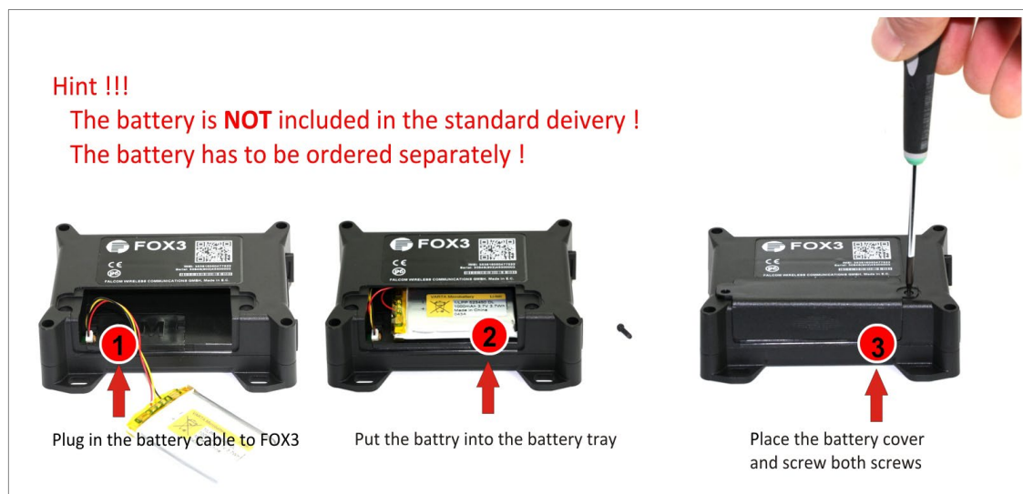
Figure 14.1: Connecting the battery to the FOX3-2G/3G/4G devices
