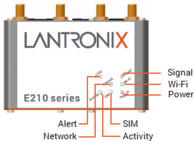
Figure 4-3: LED Status Indicators
