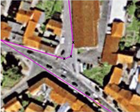
x - points in which the event "GPS.Nav.eChangeHeading2" occurs In this example, the heading tolerance is set to 22°
