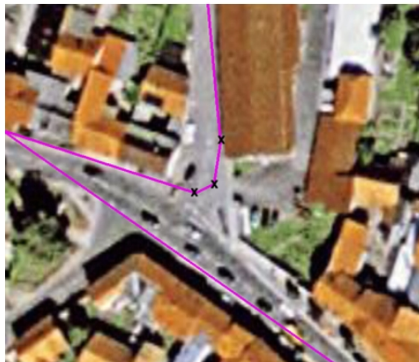
x - points in which the event "GPS.Nav.eChangeHeading" occurs In this example, the heading tolerance is set to 22°
