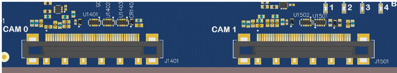
Figure 11 – MIPI CSI Camera Connectors on Rev 0200 CB
