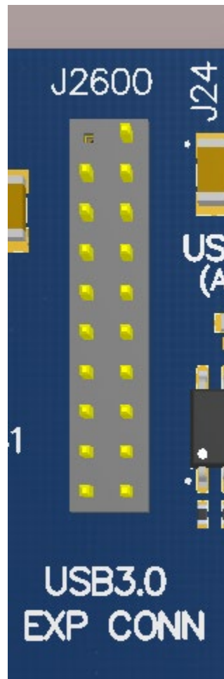
Figure 32 J2600 USB3.0 Expansion Connector
