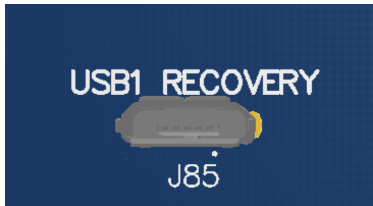
Figure 29 J85 USB1 Connector
