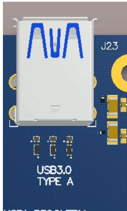
Figure 31 J23 USB3.0 Host Ports
