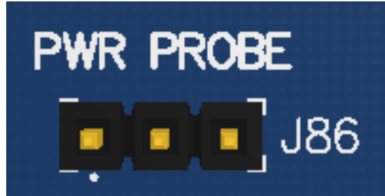
Figure 7 J86 Power Probe Header
