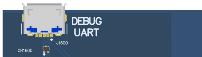
Figure 11. Debug UART over USB J1600
