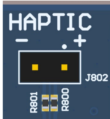
Figure 21 Haptic Motor Header (J802)
