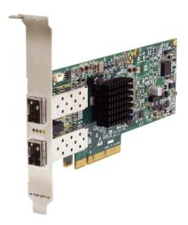
The N-TGE-SFP-01 is a 2-port PCle bus fiber NIC that supports a 1Gbps/10Gbps link. The open SFP slots can be used with 1000Base-X SFPs or 10GBase-SR/LR SFP+ modules. The NIC fully complies with IEEE 802.3ae and IEEE 802.3z standards. It provides up to 20 Gbps full-duplex bandwidth capacity to support high-end servers. It is suitable for data center, SMB and Cloud computing applications. Two LED indicators (LINK and ACT) on the bracket will help to oversee the board link and activity status.
