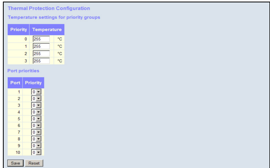
Figure 10: Configuring Thermal Protection
