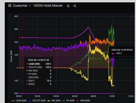
Graph view of DC microgrid during the electric grid outage
