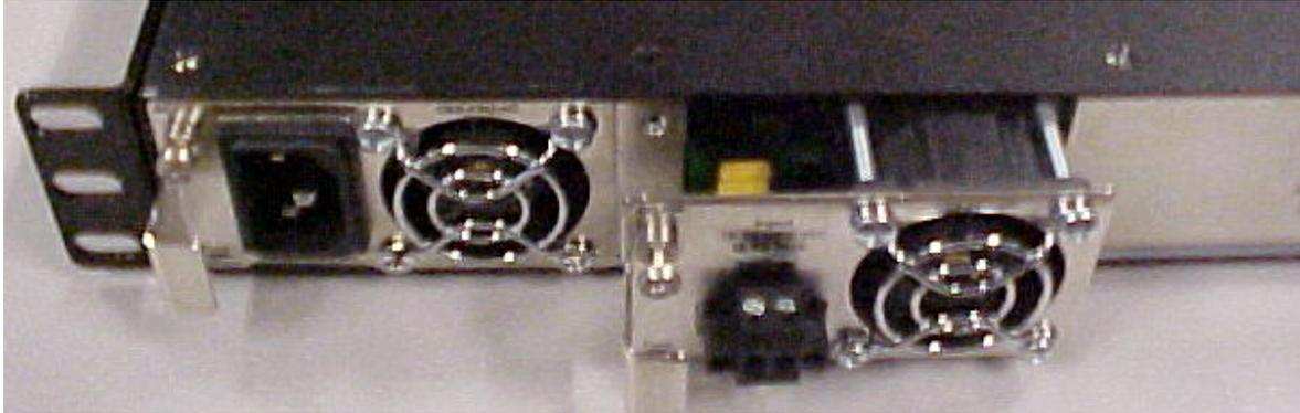
Fasten the DC Power Supply with the slotted retaining screw.
