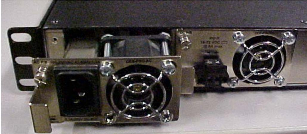
Fasten the AC Power Supply with the slotted retaining screw.
