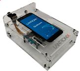
The Open-Q™ 2200 SIP is compatible with the Open-Q AL or RB development kits.
