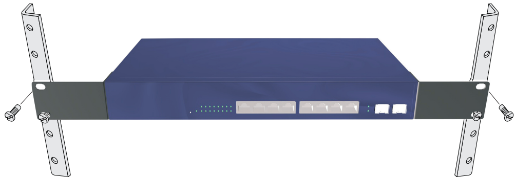
Figure 15: Installing the Switch in a Rack
