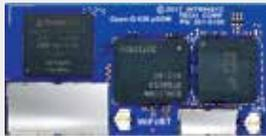
Production-ready μSOM (Micro System on Module) based on the Qualcomm® 626 processor
