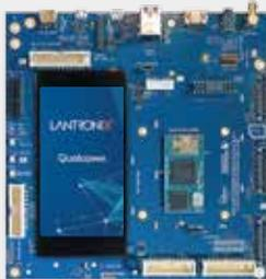
Powered by the Open-Q™ 820 μSOM (Micro System on Module)
