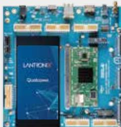
Powered by the Open-Q™ 820 SOM (System on Module)
