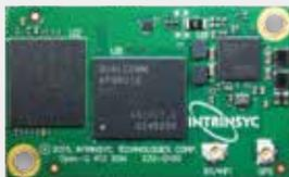
Production-ready SOM (System on Module) based on the Qualcomm® 410 processor
