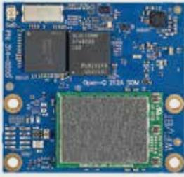
Production-ready SOM (System on Module) based on the Qualcomm® 212 processor
