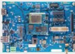
Powered by the Open-Q™ 624A SOM (System on Module)
