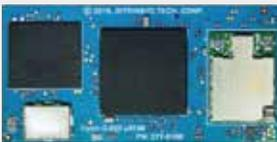
Production-ready μSOM (Micro System on Module) based on the Qualcomm® 820 processor
