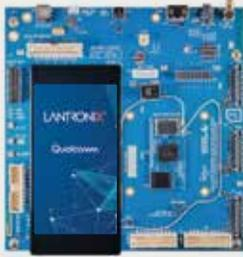
Powered by the Open-Q™ 835 μSOM (Micro System on Module)
