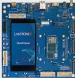
Powered by the Open-Q™ 820Pro μSOM (Micro System on Module)
