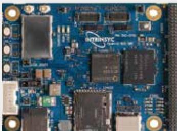
Production-ready SBC based on the Qualcomm® QCS605 System-on-Chip
