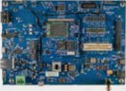
Powered by the Open-Q™ 212A SOM (System on Module)
