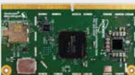
Production-ready SOM (System on Module) based on the Qualcomm® 820 processor
