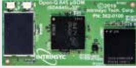
Production-ready μSOM (Micro System on Module) based on the Qualcomm® SDA845 processor
