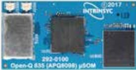
Production-ready μSOM (Micro System on Module) based on the Qualcomm® 835 processor
