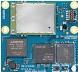
Production-ready SOM (System on Module) based on the Qualcomm® 624 processor
