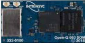
Production-ready μSOM (Micro System on Module) based on the Qualcomm® SDA660 processor
