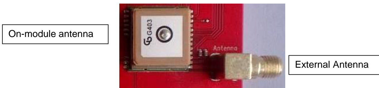
Figure 6: On-module antenna and External Antenna Connector
