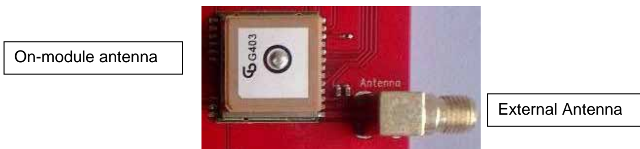
Figure 6: On-module antenna and External Antenna Connector
