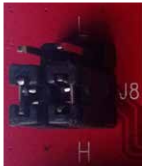
Figure 10: Configure the baud rate jumper
