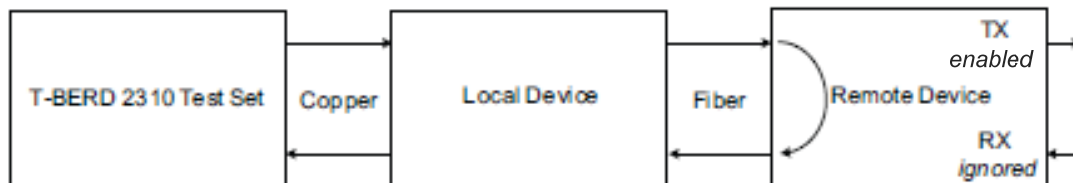
Figure 8: Initiate a Loopback from a Test Set
