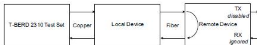
Figure 30: Initiate a Loopback from a Test Set
