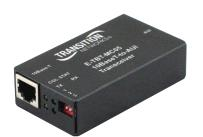
The E-TBT-MC05 is an Attachment Unit Interface (AUI) transceiver that provides a method for connecting a workstation, or any other device with an AUI port, to twisted pair cabling in a 10Base-T network. Devices with AUI ports could include: servers, hubs, bridges and routers. The E-TBT-MC05 transceiver allows twisted pair, UTP or STP, to be connected to these AUI ports.
