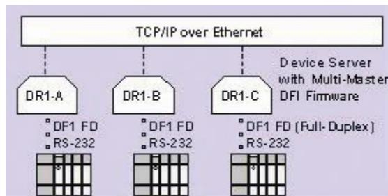
The Multi-Master DF1 firmware allows four incoming and one outgoing socket to be active at one time. This means in a simple example, that IAP Device Server-C with Multi-Master DF1 firmware can allow sockets from IAP Device Server-A, IAP Device
