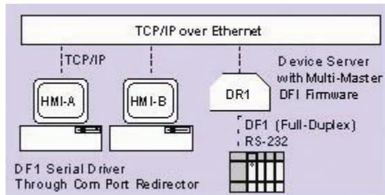
The Multi-Master DF1 firmware understands the DF1 protocol enough to prevent conflict between the masters. For example, it prevents two remote copies of RSLogix from locking the PLC resources. The first will be granted the resource, and the second will be rejected as the resource is locked already.
