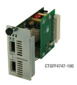
The CTGFF chassis card 10 Gigabit Ethernet fiber to fiber media converter is a (2) port 10G SFP pluggable media converter, supporting a variety of XFP and SFP+ modules. The use of these SFPs allows network designers to utilize the module to meet their network requirements.
