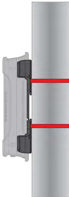
Figure 12 – Pole mount using DIN rail bracket
