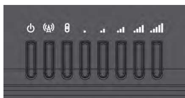
Figure 4 – NTC-220 Series router LED indicators
