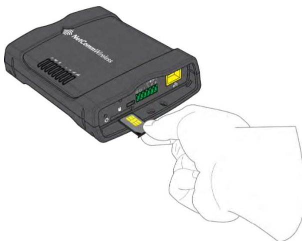
Figure 17 – Inserting the SIM card
