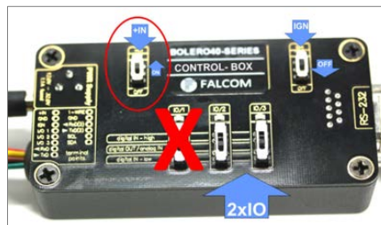
Figure 7: Overview of the control-box top panel (IGN = ON)
