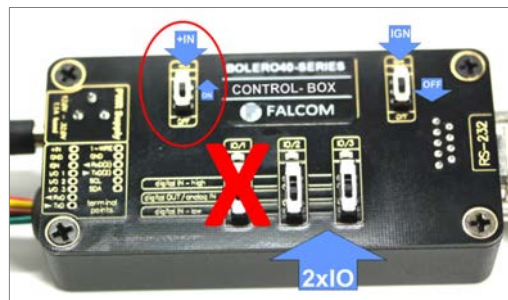
Figure 5: Overview of the control-box top panel (+IN = ON)
