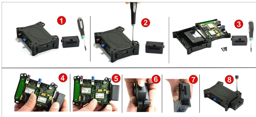
Figure 4 – Connecting IOBOX-mini to FOX Series device
