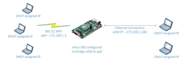
In this configuration, the ap0 interface acts as the DHCP server for any wireless bridged devices, and eth0 acts as the DHCP server for wired devices.
