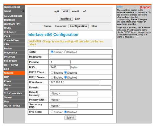
Figure 5: Configuring eth0 to allow for static IP address bridge capability.
