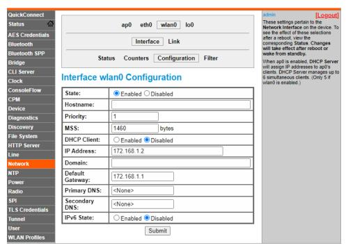
Figure 4: Configuring wlan0 to allow for static IP address bridge capability.
