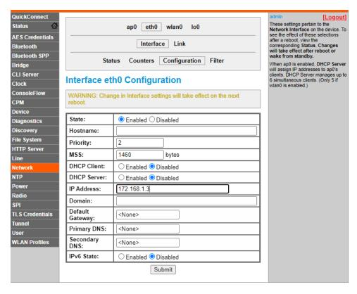
Figure 3: Configuring eth0 to allow for static IP address bridge capability.
