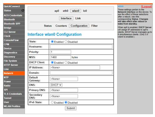
Figure 8: Configuring wlan0 to allow for DHCP address bridging.
