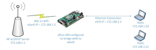
In this scenario, the static IP address configuration allows the xPico 200 to act as a simple network bridge where IP addresses must be on the same subnet. Multiple bridged devices are supported.
