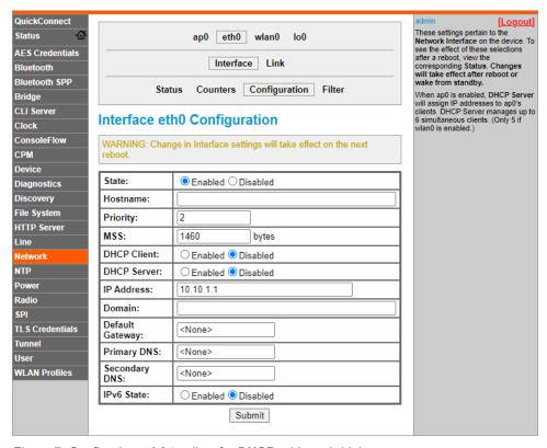
Figure 7: Configuring eth0 to allow for DHCP address bridging.
