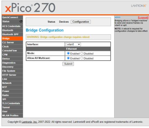
Figure 1: Enabling wlan0 bridge mode in the xPico 270 configuration.
