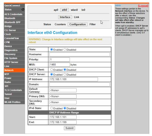
Figure 9: Configuring eth0 to enable DHCP bridging.
