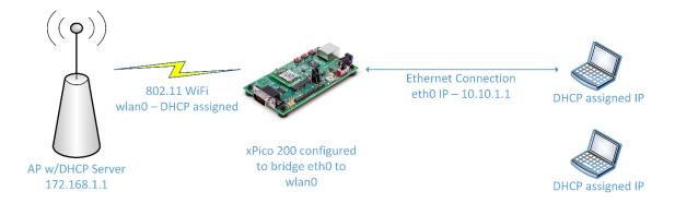
In this scenario, the DHCP server is in the wlan0 network. The xPico 200 will forward DHCP requests from bridged devices to the wlan0 DHCP server. Multiple devices are supported.
