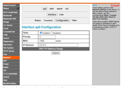
Figure 6: Configuring ap0 to allow for static IP address bridge capability.
