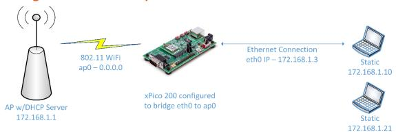
In this scenario, multiple bridged devices can communicate with the xPico 200 on the eth0 interface. Assigning IP address "0.0.0.0" to the ap0 interface will disable network services over ap0, including the DHCP server. All other IP addresses must be on the same subnet.
