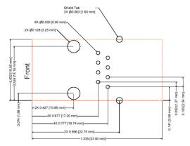
For proper heat dissipation, the PCB should have approximately 1 square inch of copper attached to the shield tabs. The shield tabs are an important source of heat sinking for the device.
