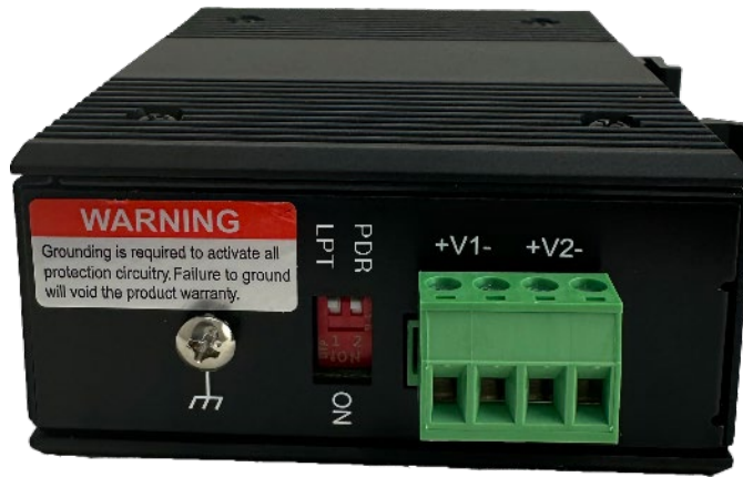
Figure 2-4 Power Input with 4-pin terminal block
