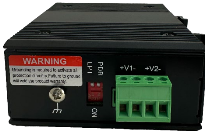
Figure 2-4 Power Input with 4-pin terminal block
