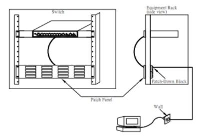
**Network Wiring Connections**
