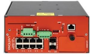
The LSS2200-8P is a managed Layer 2+ Gigabit Ethernet switch offering eight (8) 1GBase-T interfaces with full IEEE 802.3bt 90W support, two (2) 10/5/2.5/1GBase-T multi-gigabit SFP+ slots, two (2) programmable Digital Input/Outputs with 12V power output, and one (1) RJ-45 console port. The switch offers 720W total PoE budget for powering LED lighting, high-powered security and surveillance cameras and other IP devices.
