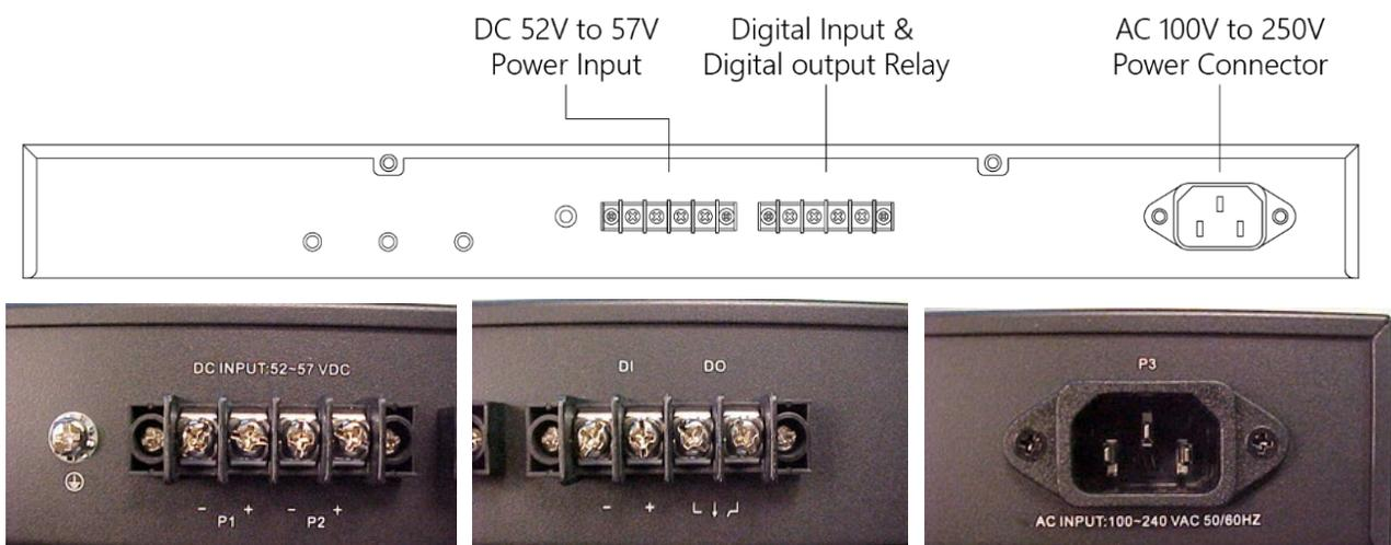
**Install the Switch:** **Note** that if you must use the switch to connect outdoor devices such as outdoor IP cameras with cable, then you must install an arrester on the cable between outdoor device and the switch.
