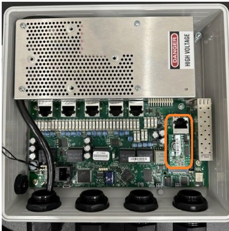
SESPM1040-541-LT-AC with Installed SESPM-2P-24V-CP 24V Passive PoE Port Module
