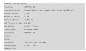
**Initial Switch Config via CLI**: Access the Command Line Interface via telnet or SSH. See the *CLI Reference*.
